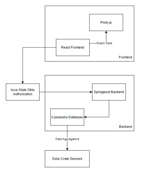
We will have a React-based frontend that interacts with a Spring Boot backend. Our data is stored within a Cassandra database, which grabs data from the microgrid via Python script data aggregators.
