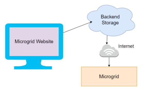
Our web application's design consists of a frontend and backend, along with the physical ISU EPRC Solar Crate. The backend communicates with sensors on the Solar Crate to store information about efficiency and power usage on the cloud, which is then displayed by the frontend of the website for users to see and interact with.
